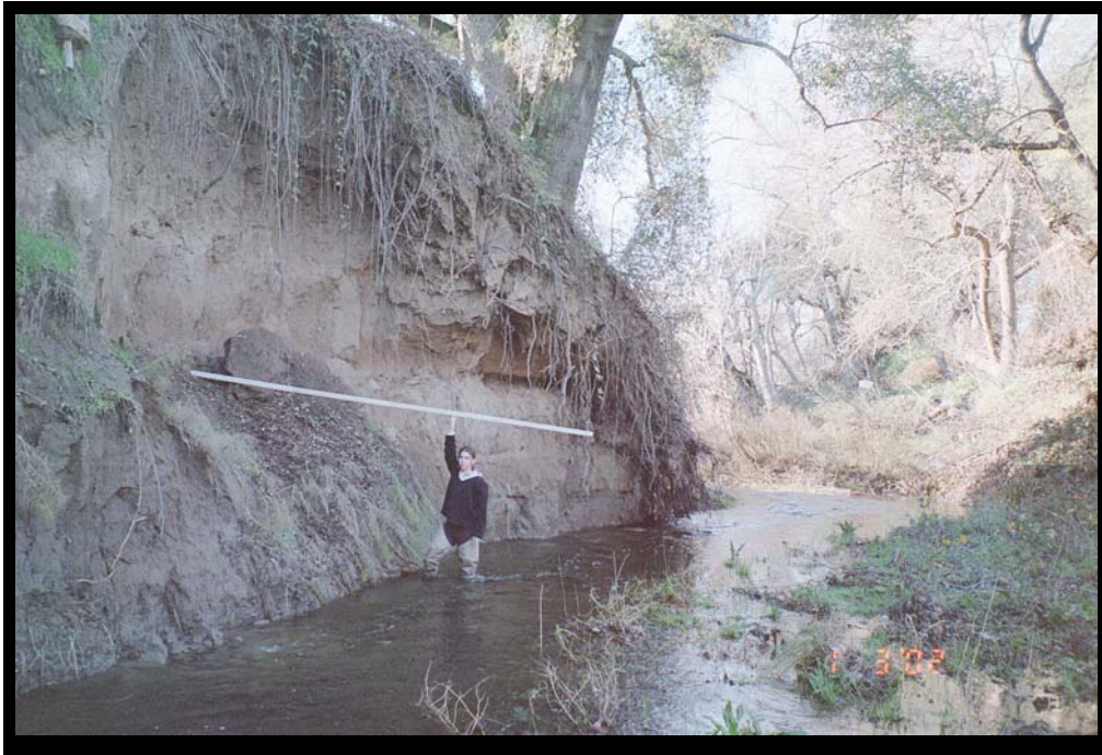
Stream channel erosion caused by excessive urban runoff and the loss of native vegetation. Location: Atascadero Creek
